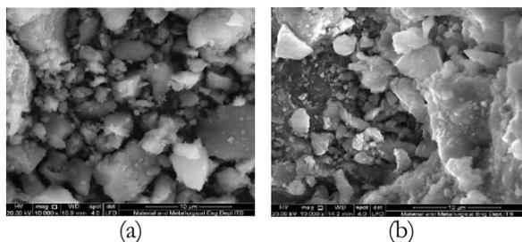
Fig 2. SEM analysis with 10,000x magnification (a) Chi-FA-Fe<sub>3</sub>O<sub>4</sub> composite and (b) Chi-FA-Fe<sub>3</sub>O<sub>4</sub> composite after adsorption of CR dye
