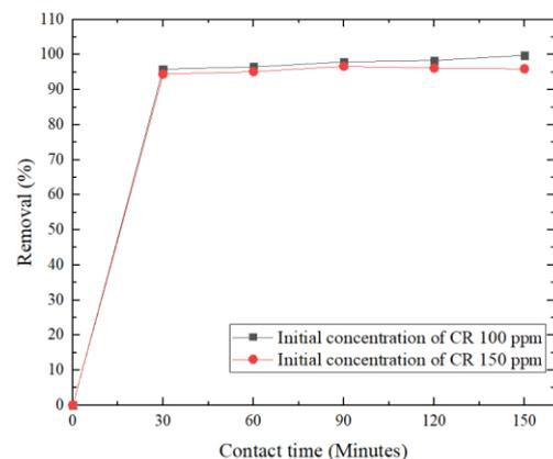
Fig 3. Effect of contact time and initial dye concentration on the adsorption of CR dye with Chi-FA-Fe<sub>3</sub>O<sub>4</sub> composite adsorbent
