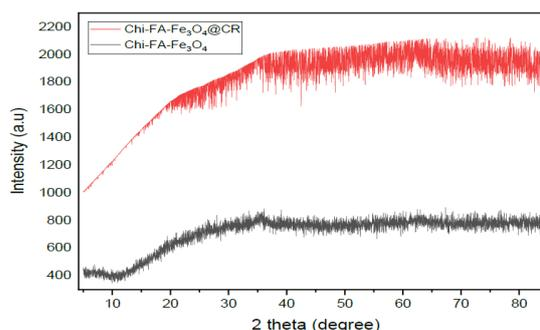
Fig 1. XRD analysis of Chi-FA-Fe<sub>3</sub>O<sub>4</sub> composite adsorbent and Chi-FA-Fe<sub>3</sub>O<sub>4</sub> composite after CR dye adsorption
