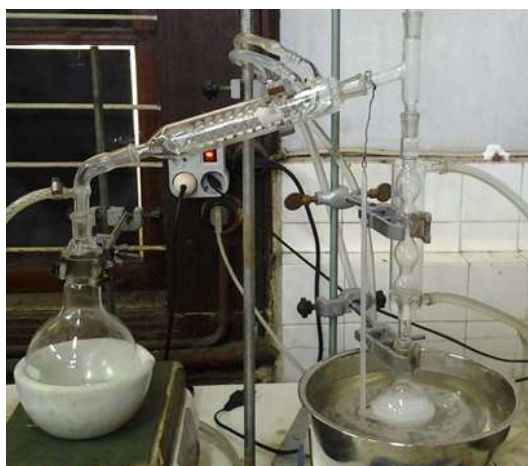
Fig. 2. Sol-gel reaction with reflux treatment set-up, consist of: mixing stirrer, hotplate, distillation tube and vacuum system.
